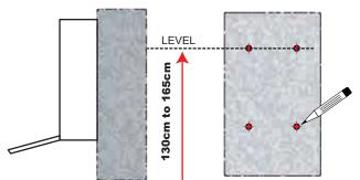
3 Using the 4mm drill bit provided, create four pilot holes at least 10mm deeper than screws provided, or about 40mm deep. If the material is unusually hard you may need to use a rotary impact drill rather than a standard drill to make the holes. Call a handy man if needed. Put a small amount of caulk or silicone
